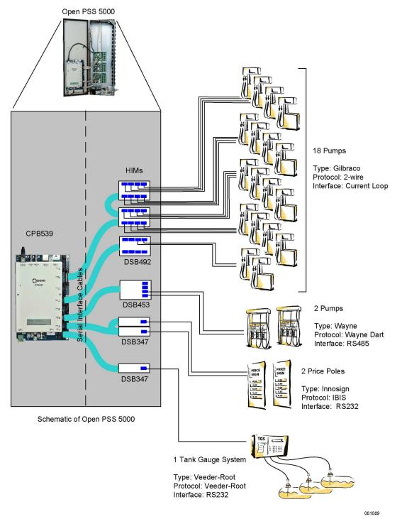
**Note:** This illustrates that only 16 devices using the Current Loop interface can be connected to a single port (2 of the DSB492 HIMs are daisy chained together and connected to a single port). Under normal circumstances, we recommend that load balancing is used on the ports when connecting multiple devices (with the same protocol) to multiple modules – this increases performance.
