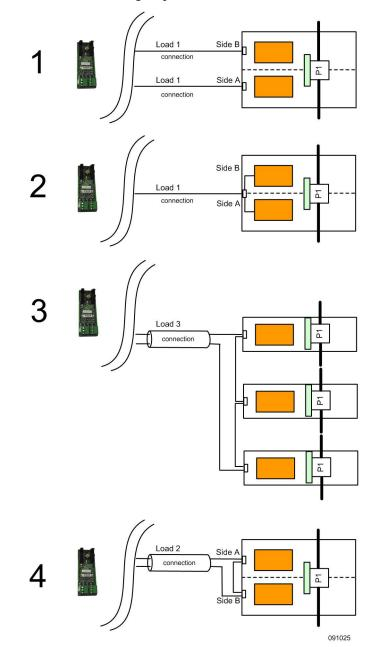
Example 1 represents a dual-sided dispenser, where each dispenser is a device and each device requires a connection to the HIM. In this situation, the load on each HIM connection is 1 device.
